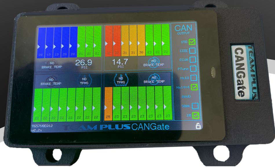
Display and connect Team Plus<sup>®</sup> sensors to your existing CANbus dash logger using the Team Plus<sup>®</sup> CANGate<sup>®</sup>. CANGate<sup>®</sup> connects to the Team Plus<sup>®</sup> Wheel Turtle<sup>®</sup>, Team Plus<sup>®</sup> TPMS and Team Plus<sup>®</sup> Brake Turtle<sup>™</sup>(\*) sensors over Bluetooth and then passes data onto your CANbus, so it is available to any CAN based dash or logger or ECU.
