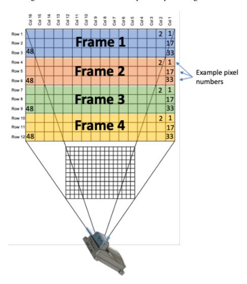
4 messages (frames) sent per update, 1 per frame. Utf-8 comma delimited strings are notified for each message contains a header code and pixel heat values in degrees Celsius.
